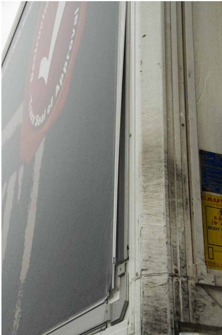
Test 3 The horizontal frame is re-clipped and the lower corner cover plate removed. 1 meter of the vertical frame rail was unclipped from the lower corner.
