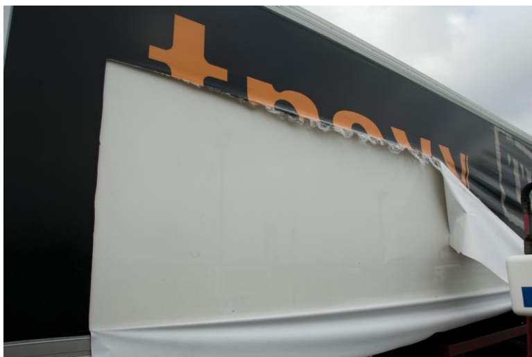
Test 15 The sign material was physically torn rearwards from the knife cut to emulate typical vandalism.
