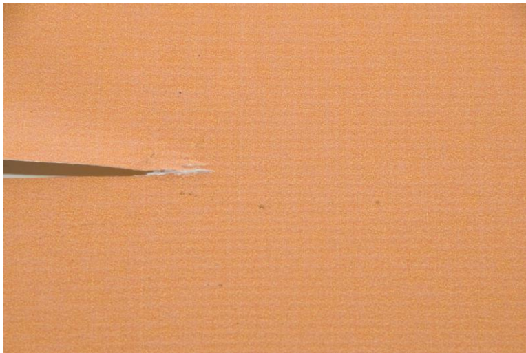
Test 9 12 mm tear at the end of the horizontal cut with 10 mm delaminating of the material surface coating
