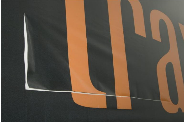
Test 10 The horizontal cut extended to a length of 2 meters
