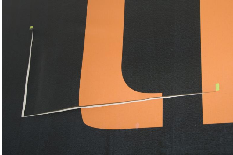
Test 9 Vertical cut for 500 mm from the front of the 1 meter horizontal cut
