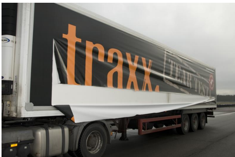
Test 13 The sign was cut for the full length of the trailer.
