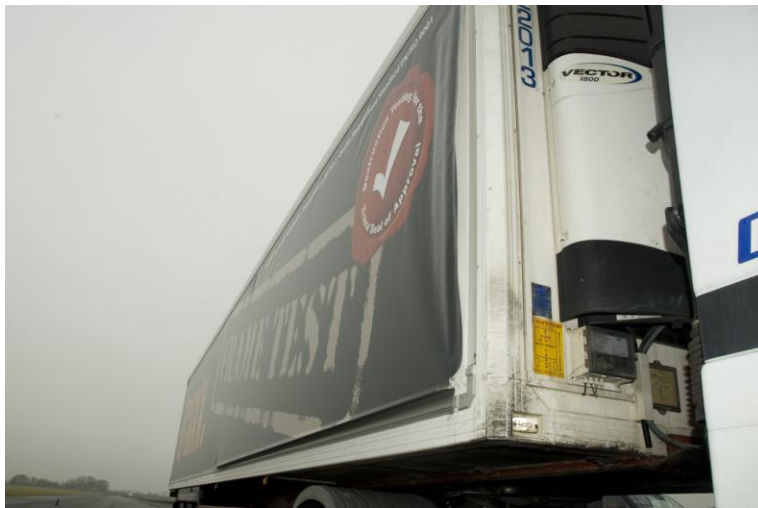
Test 6 The horizontal lower frame was un-clipped and the vertical rail was not refitted.
