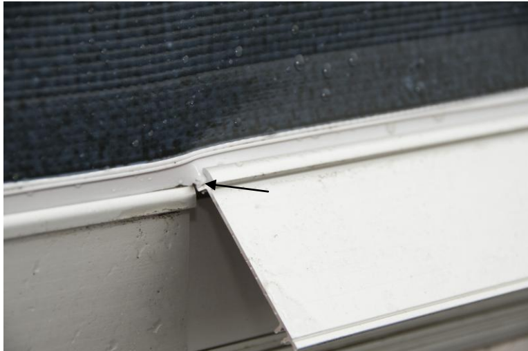
Test 2 Tear in the lower plastic section of the sign mounting system
