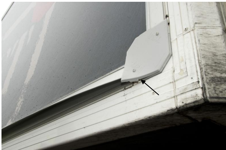
Test 2 Lower corner cover plate retaining the horizontal frame rail after test.
