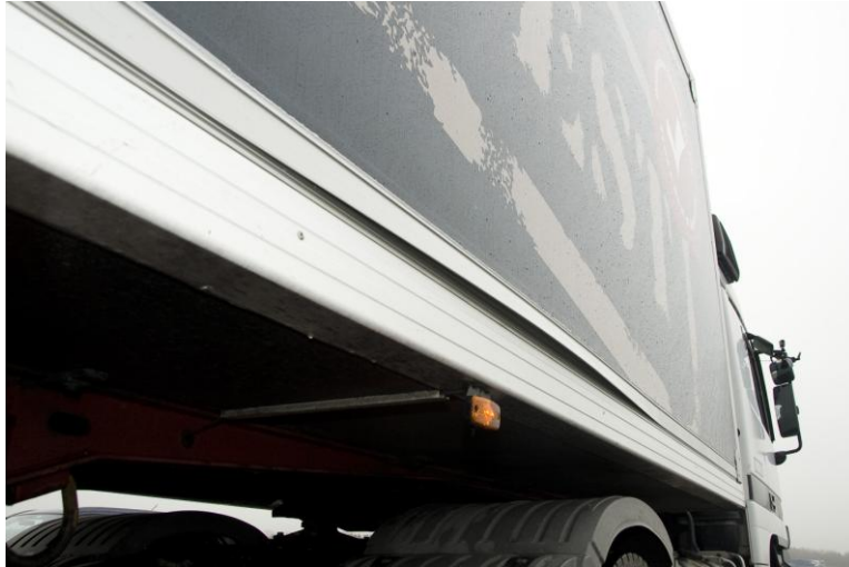
Test 1 Horizontal frame unclipped for 2 meter, 2 meter back from the vertical frame
