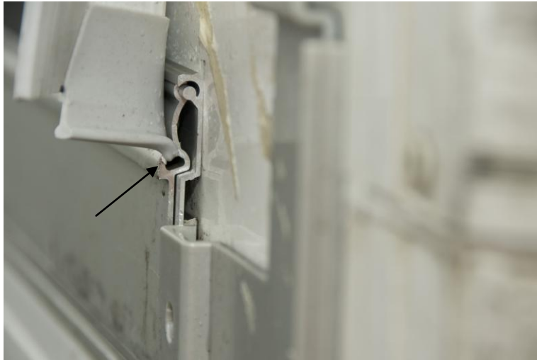
Test 5 After completing two laps the plastic lower moulding for the sign was trapped in the lower horizontal rail.
