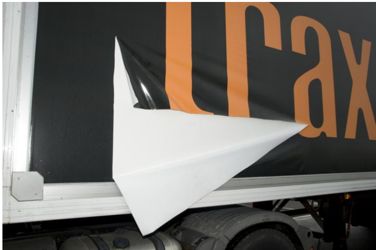
Test 11 The vertical cut was extended down to the lower horizontal frame rail
