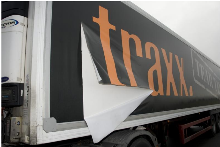
Test 12 The vertical cut was extended by 500 mm to a length of 1.5 meters
