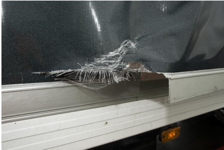
Test 6 The sign material tore at the attached rear lower horizontal frame
